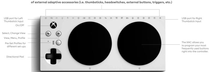
The Xbox Adaptive Controller has 20 different 3.5mm jacks that allow you to connect a variety of external adaptive accessories (i.e. thumbsticks, headswitches, external buttons, triggers, etc.
